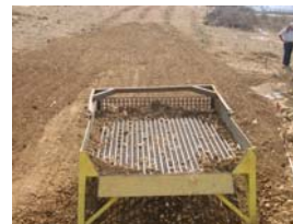
Locally manufactured “sifter” to assist with clearance of large piles of bulldozed spoil containing Anti Personnel mines
